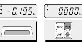
(1) Remove the container and commodity, then the display will show the weight of the container with "-" sign.
